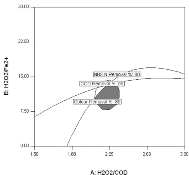
FIGURE 5. Overlay plot for optimal region at reaction time 1.5 h
