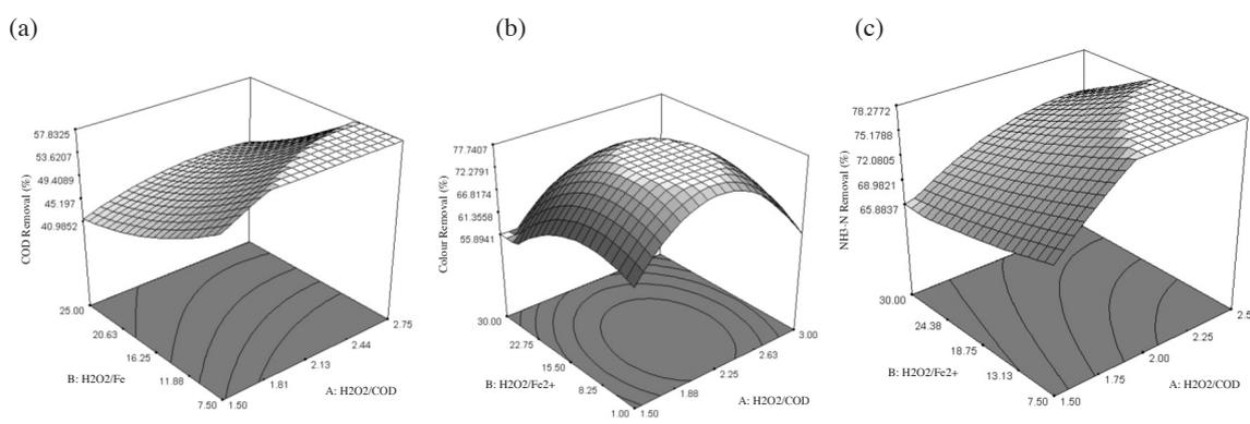
FIGURE 4. Response surface plot of (a) COD, (b) Colour & (c)  $\text{NH}_3\text{-N}$  removal as function of  $\text{H}_2\text{O}_2/\text{COD}$  molar ratio and  $\text{H}_2\text{O}_2/\text{Fe}^{2+}$  molar ratio at reaction time 1.5 h
