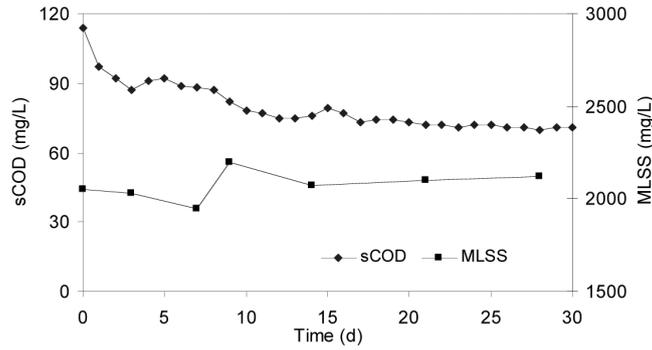
FIGURE 6. Effluent soluble COD (sCOD) & MLSS in SBR
