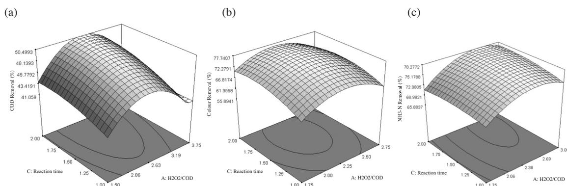
FIGURE 2. Response surface plot of (a) COD, (b) colour & (c) NH<sub>3</sub>-N removal as function of H<sub>2</sub>O<sub>2</sub>/COD molar ratio and reaction time at H<sub>2</sub>O<sub>2</sub>/Fe<sup>2+</sup> molar ratio 20
