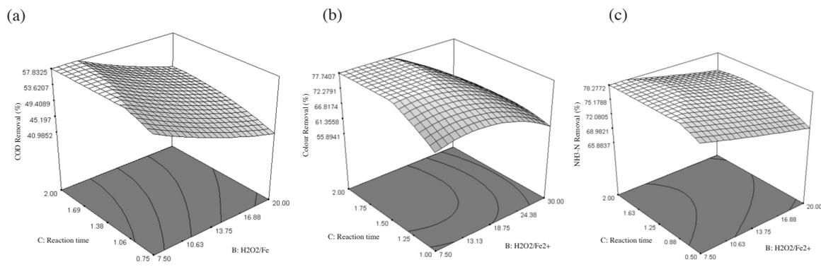
FIGURE 3. Response surface plot of (a) COD, (b) colour & (c)  $\text{NH}_3\text{-N}$  removal as function of  $\text{H}_2\text{O}_2/\text{Fe}^{2+}$  molar ratio and reaction time at  $\text{H}_2\text{O}_2/\text{COD}$  molar ratio 2.0
