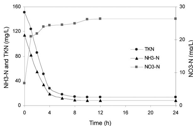
FIGURE 9. Ammonia-nitrogen (NH<sub>3</sub>-N), nitrate-nitrogen (NO<sub>3</sub><sup>-</sup>-N) & total Kjeldahl nitrogen (TKN) in SBR during 24 h cycle
